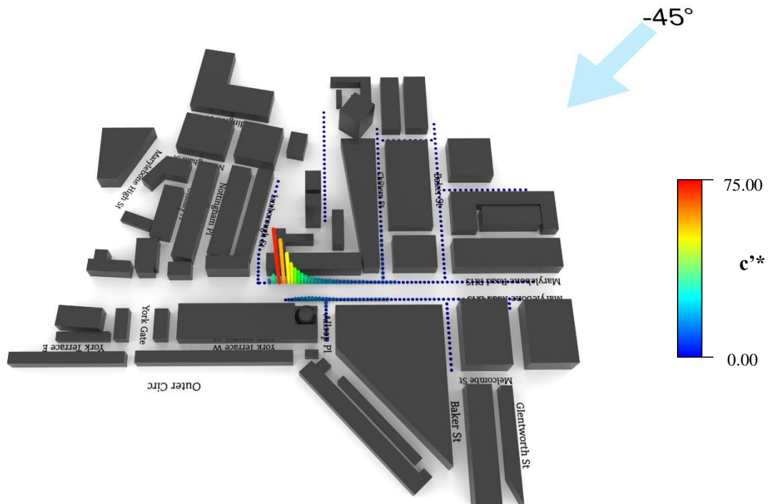
Figure C2: 3D plot of non-dimensional standard deviation of concentration fluctuations, c'^* from forward modelling at a wind direction of -45^\circ with varied source release location and fixed FFID at (202.5, -74, 10) mm
